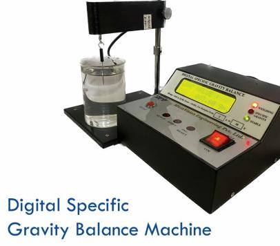
A specific gravity balance is used to measure the buoyancy of an object by weighing that object in air and then in water.
