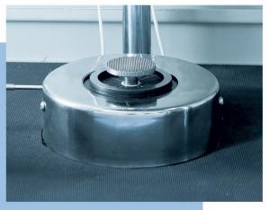
It is an instrument consisting of a motor driven disk within a die cavity formed by two dies maintained at specified conditions of temperature and die closure force. It measures the effect of temperature and time on viscosity of rubber or compound.
