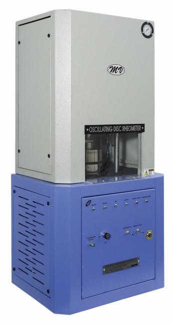
Oscillating Disc Rheometer shows a typical Cure Curve obtained in the software test screen. The curve of Torque V/s Cure Time depicts all the vulcanization characteristics of the Rubber Compound and that can be determined directly. XY Plot of Torque (F) against real cure time is called Rheometer graph. Rheometer graph is displayed in real time and at the end of test time, software and displayed on the screen.
